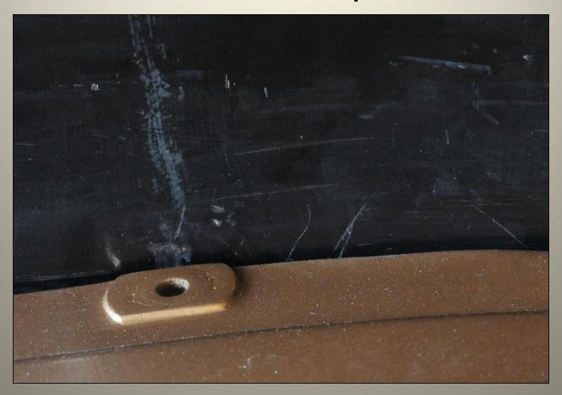
On some pianos you will need to create a counter bore so the top of the perimeter bolt can be flush to the soundboard
