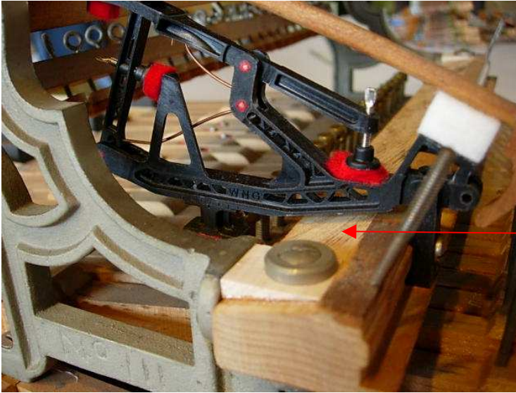
Fig. 10 Repetition rail re- installed with proper clearance
