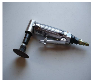
Fig. 2 Right angle die grinder W quick-change disc holder for 2" discs
